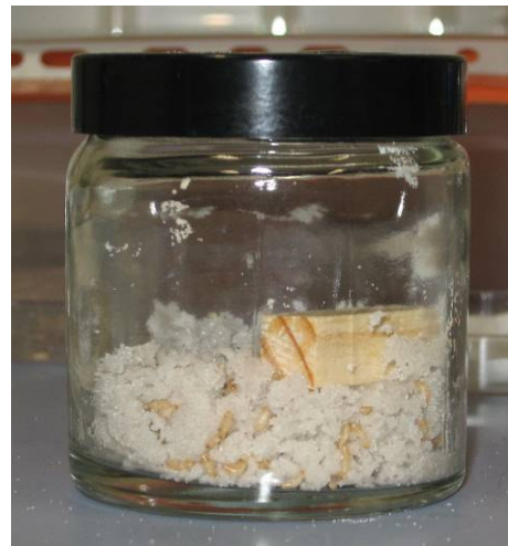
Figure 4 – a completed test container with visible the humid sand, the wood sample, and the workers
