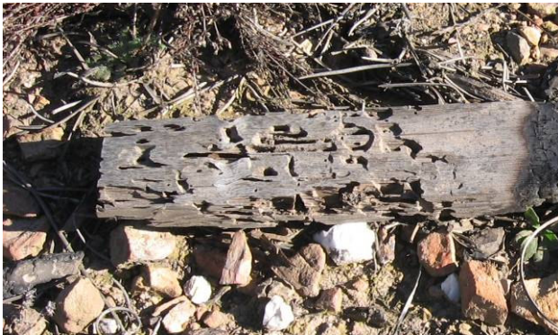
Figure 1 – a stake with visible signs of termite attack
